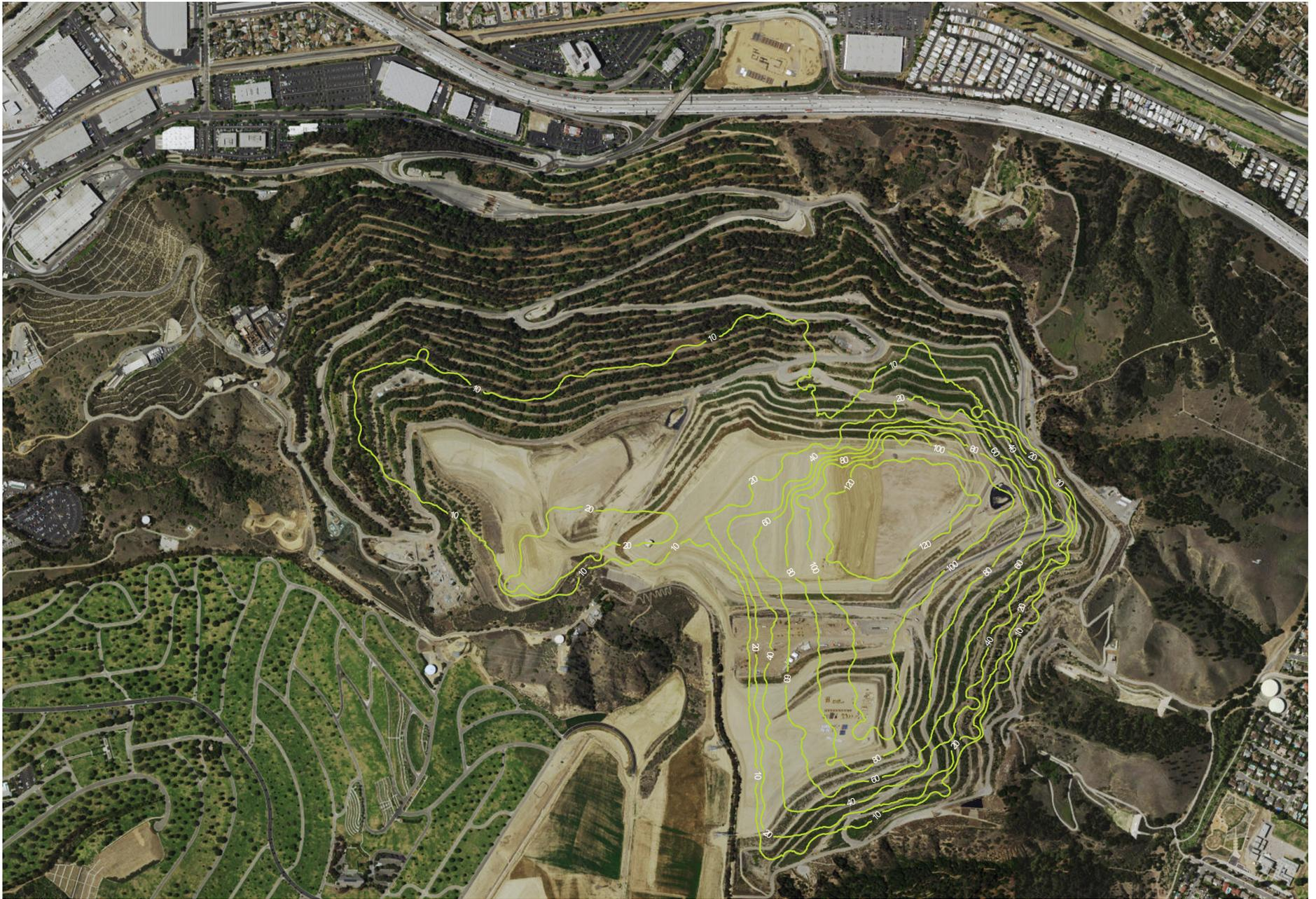
**LANDFILL SETTLEMENT PROJECTION (ISO-SETTLEMENT CONTOURS).** THIS EXHIBIT SHOWS THE ESTIMATED AMOUNT OF SETTLEMENT IN FEET, WHICH WILL OCCUR OVER A 30-YEAR PERIOD. THE EASTERN DECK WHICH CONTAINS THE DEEPEST FILL AREA, WILL SETTLE THE MOST—APPROXIMATELY 125 FEET IN 30 YEARS.
