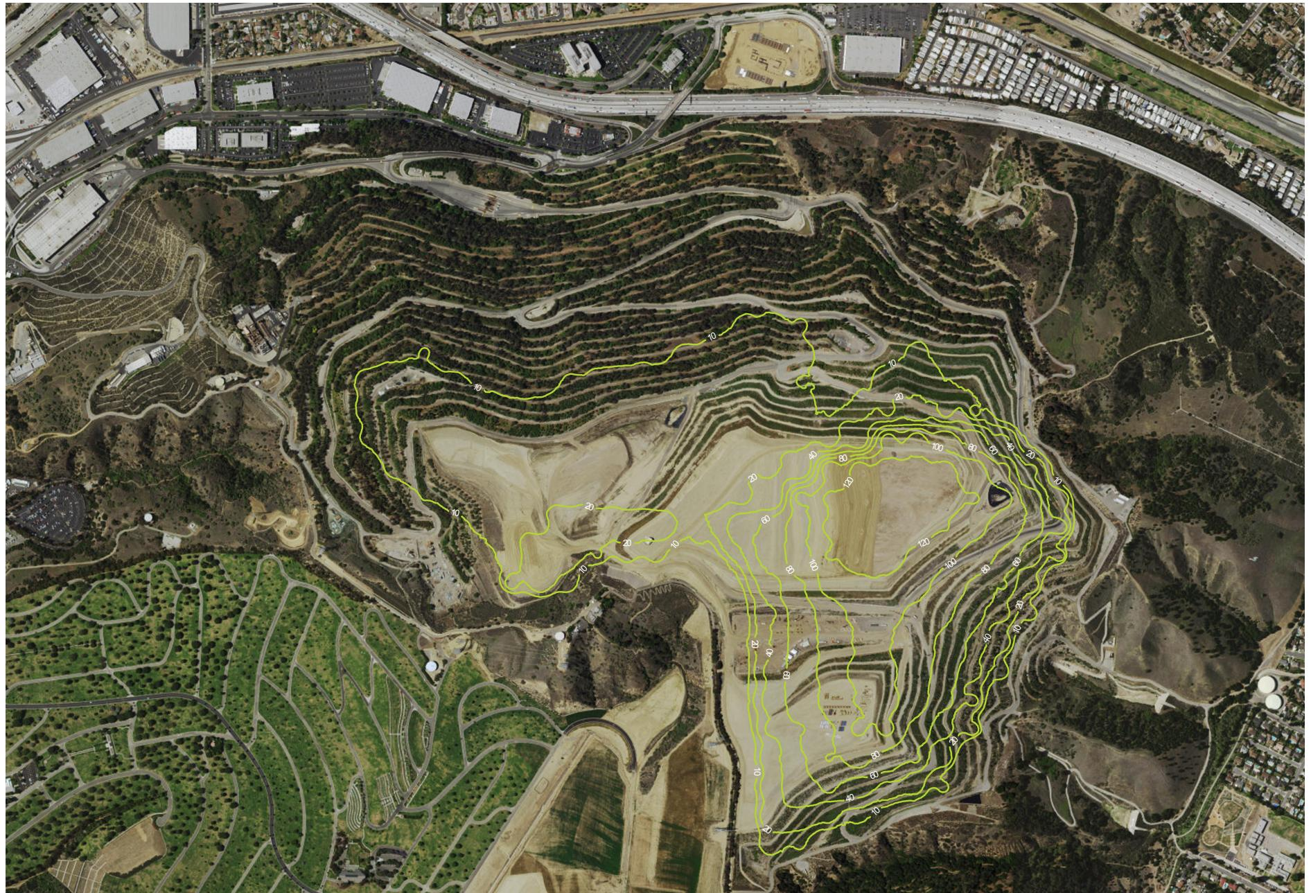
**LANDFILL SETTLEMENT PROJECTION (ISO-SETTLEMENT CONTOURS).** THIS EXHIBIT SHOWS THE ESTIMATED AMOUNT OF SETTLING IN FEET, WHICH WILL OCCUR OVER A 30-YEAR PERIOD. THE EASTERN DECK WHICH CONTAINS THE DEEPEST FILL AREA, WILL SETTLE THE MOST—APPROXIMATELY 125 FEET IN 30 YEARS.
