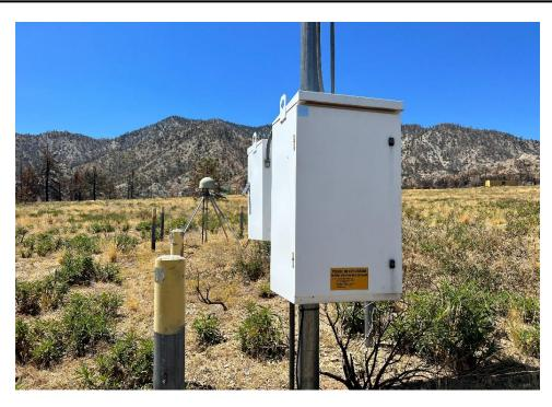
Photograph 11: View of seismic monitoring system located in the vicinity to the west of the site.
